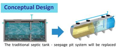
The traditional septic tank - seepage pit system will be replaced with a fixed-film aeration tank to prevent subsidence of the ENO4 building. This upgraded system is not only more efficient but also contributes to environmental sustainability.
